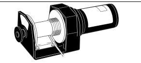
Fig. 5 Never Operate Winch with Less Than Five Turns Around Drum
